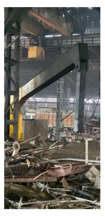
We are manufacturers of Hydraulic Pusher and delivers to several steel industries for induction furnace as per their requirements. Hydraulic Scrap Pocker mainly used to push the scrap into the induction furnace during the melting operation in the steel foundries. Hydraulic Pusher functionality is column-mounted and control through remote.
