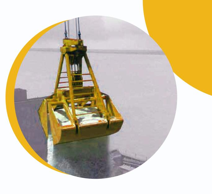
Four Rope Mechanical Clamshell Grabs for attachment to four line operated cranes. (Two Holding Ropes and Two Closing Ropes). The grabs are specially designed for charging and discharging sand, gravel and other bulk materials. The grabs can be executed with open or closed shells depending on the job and the type of material to be handled. The grabs are manufactured of high wear resistant steels. All bearings are heavy-duty and sealed for high performance.
